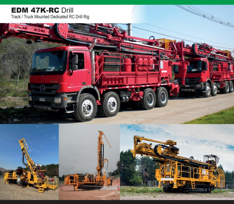
The EDM47K-RC is a versatile dedicated reverse circulation drill with 47,000lbs of pullback capacity. The drill is designed to be easily customized and can be truck or track mounted with multiple engine, cyclone, splitter, and breaker options available enabling the end user to tailor the rig according to their unique requirements.
