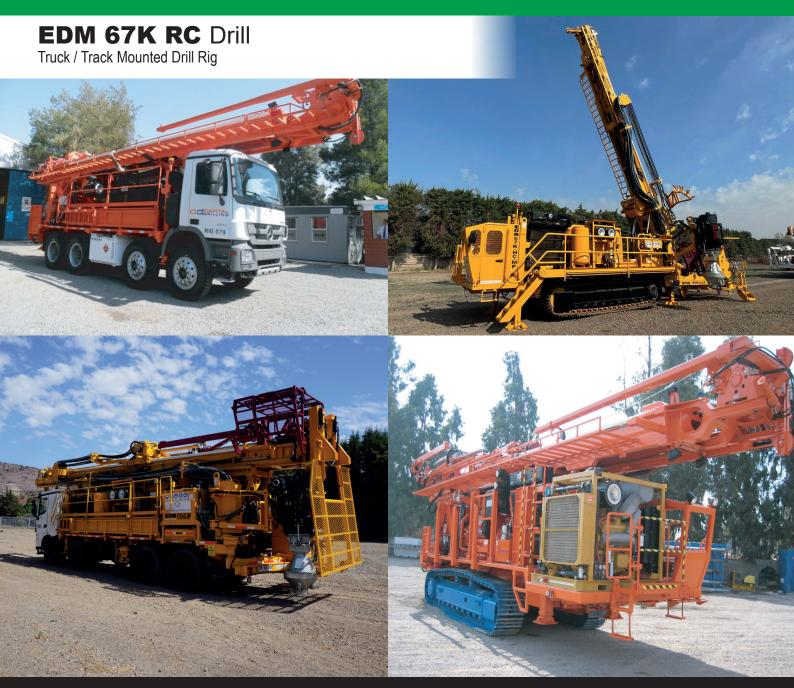
The EDM67K-RC Drill is a heavy duty dedicated reverse-circulation machine with a proven track record for deep exploration projects in challenging environments. The rig has 67,000lbs pullback capacity, can be truck or track mounted and comes with all the safety features required for working on Tier 1 mine sites.
