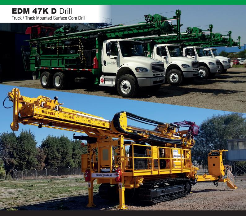
The EDM47K-D Drill is a mid-size surface core drill with 47,000lbs of pull back capacity and capable of drilling to more than 2000m in tough environments. The rig features a robust 2 speed top drive rotation head delivering 1250rpm and 6,713Nm of torque, deck engine options up to 400HP, a 40,000ll capacity main winch and can be delivered track or truck mounted, or ready to mount to customers own vehicle.
